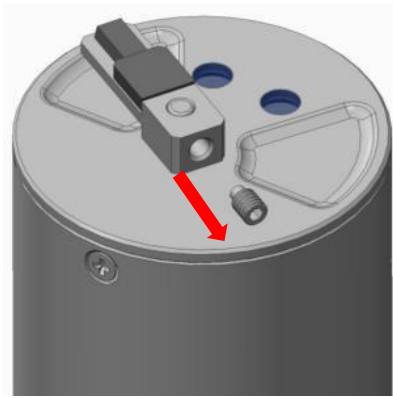
Figure 30 Remove the M2 screw
