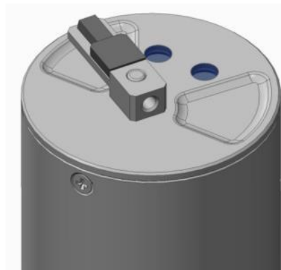
Figure 32 Install the new wiper arm
